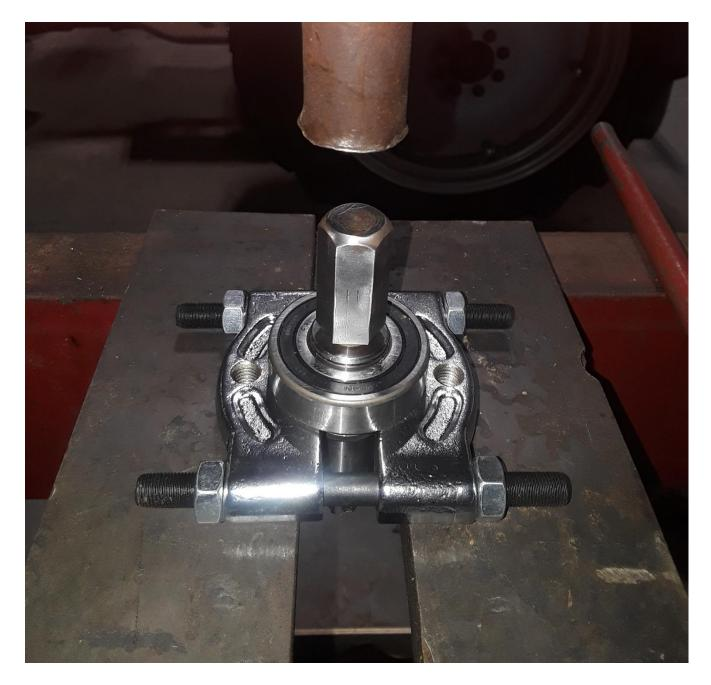
3.9. Install the shaft spacer followed by the inner bearing race on to the shaft by pressing them on from the splined end of the shaft.
