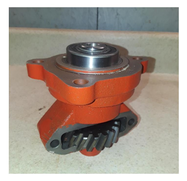
3.11. Assemble the pump adapter plate to the gear housing using a new gasket and four 3/8 x 1" socket head cap screws. Do not fully tighten the screws until you complete the next step.
