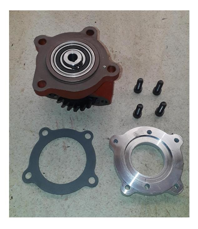
3.12. Finally assemble the pump to the adapter plate using a new gasket and two 3/8 x 1<sup>°</sup> socket head cap screws. The narrow side of the pump housing should be clocked to the gear opening side of the housing. Evenly tighten all six socket head screws to 20 lb-ft.
